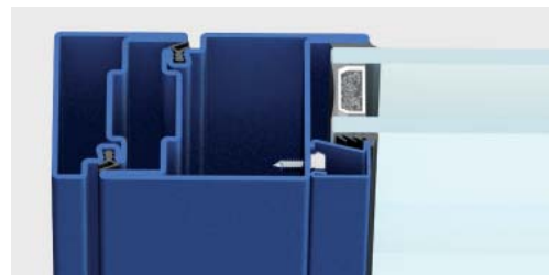
reduced lateral section | frame section 106 mm
