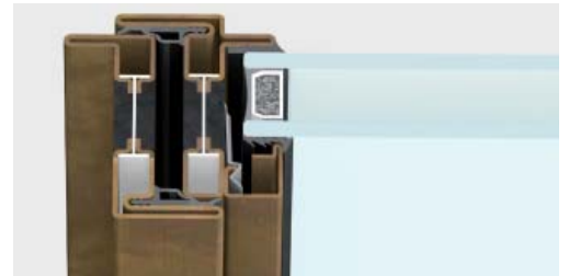
lateral section | frame section 47 mm
