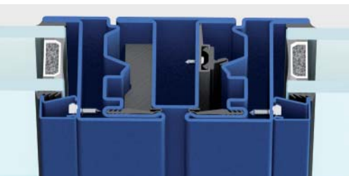
central section | rebated | frame section 145 mm
