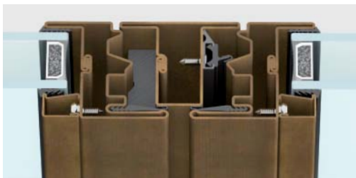
central section | rebated | frame section 145 mm
