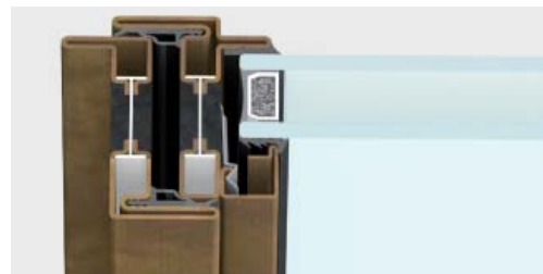
lateral section | frame section 47 mm
