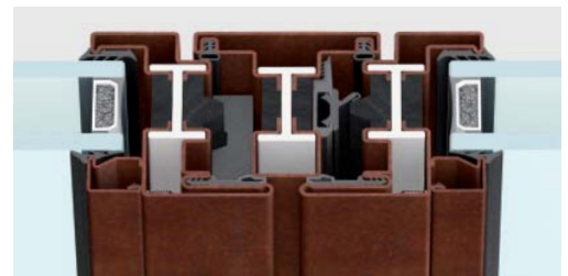
double-sash window central section* | frame section 145mm
